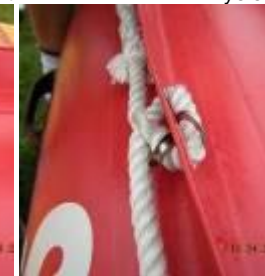
Eyelet is broken – cut hazard (see above and below)
