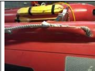
Life line is too tight:
