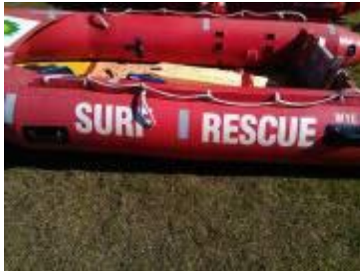
Sufficient slack (but not too much): Eye lets in good condition, not lifted and not sharp or corroded
