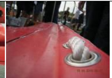
Eyelet has lifted – potential cut hazard
